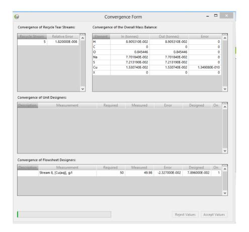
f. During the calculation, the progress will be shown. Once the mass balance tolerances have been achieved the calculation will stop.
