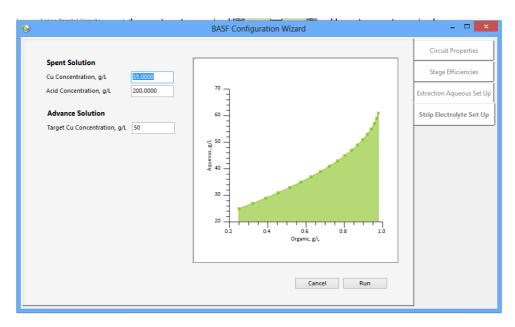
e. Once this is complete you can "Run" the balance. The wizard will first configure the mass balance to the parameters you have specified and then calculated the closed mass balance for the specified circuit.
