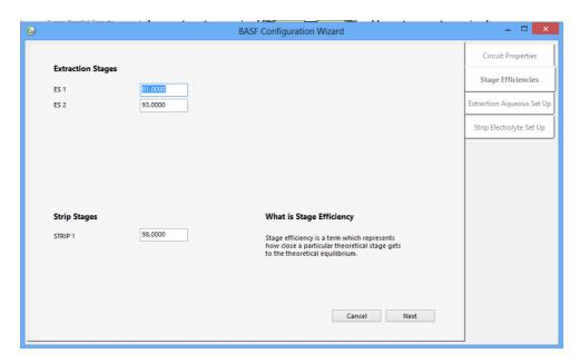
c. After stage efficiencies, configure the PLS stream(s). If you have more than 1 PLS stream then you must configure each stream before moving on. If they have the same composition then you can select the check-box telling Isocalc<sup>TM</sup> to make them all the same.
