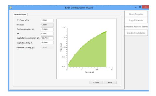
d. After that, define the strip conditions. Here you must specify the spent copper concentration, the acid concentration and the exit copper concentration. Isocalc will determine the required spent flowrate to achieve the delta across the strip.
