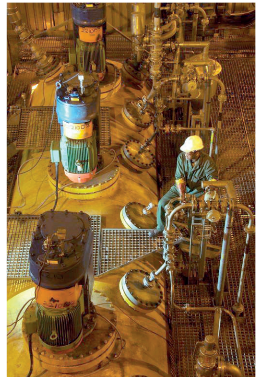
Figure 1: A pressure leaching autoclave (Crundwell, et al., 2011, photo courtesy of M. Fox).
